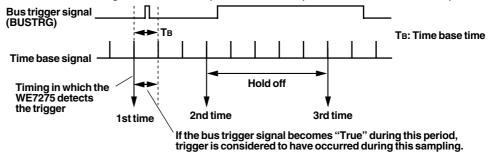
In addition, the WE7275 can output a bus trigger signal upon detecting a trigger within the module, and receive the results of the AND/OR computation on the bus to trigger the actual trigger operation.
